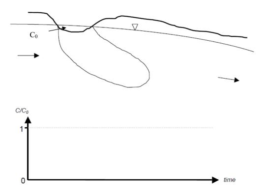
b) Advection and dispersion (happening in all directions). In this case the heavy solid line indicates  $C/C_0$  of 0.5.
